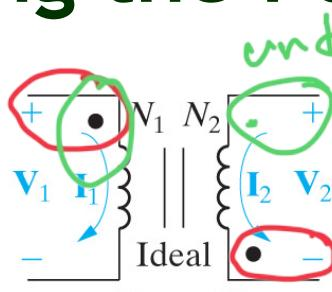
$$\frac{V_1}{N_1} = \frac{V_2}{N_2}, \\ N_1 I_1 = N_2 I_2$$
