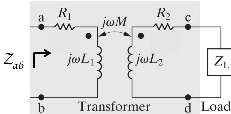
$$Z_{ab} = \underbrace{\mathcal{R}_1 + \frac{\omega^2 \mathcal{M}^2 (\mathcal{R}_2 + \mathcal{R}_L)}{(\mathcal{R}_2 + \mathcal{R}_L)^2 + (\omega \mathcal{L}_2 + \mathcal{X}_L)^2}}_{\mathcal{R}_{ab}} + j \underbrace{\left( \omega \mathcal{L}_1 - \frac{\omega^2 \mathcal{M}^2 (\omega \mathcal{L}_2 + \mathcal{X}_L)}{(\mathcal{R}_2 + \mathcal{R}_L)^2 + (\omega \mathcal{L}_2 + \mathcal{X}_L)^2} \right)}_{\mathcal{X}_{ab}}$$
