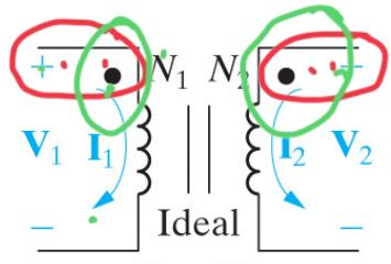
$$\rightarrow \frac{V_1}{N_1} = \frac{V_2}{N_2}, \\ N_1 I_1 = -N_2 I_2$$
