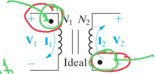
$$\frac{V_1}{N_1} = -\frac{V_2}{N_2}, \\ N_1 I_1 = -N_2 I_2$$
