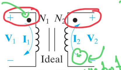
$$\frac{V_1}{N_1} = \frac{V_2}{N_2}, \\ N_1 I_1 = N_2 I_2$$
