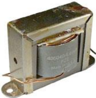
4mH high-current choke
