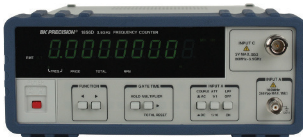
FIG. 13.79 Frequency counter, 3.5 GHz multifunctional instrument. (Courtesy of B+K Precision)
