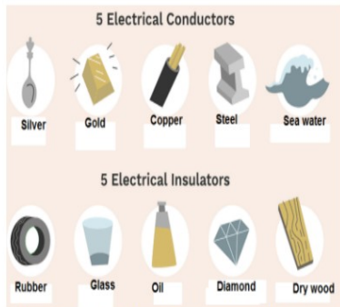
Figure 10: Examples of conductors and insulators
