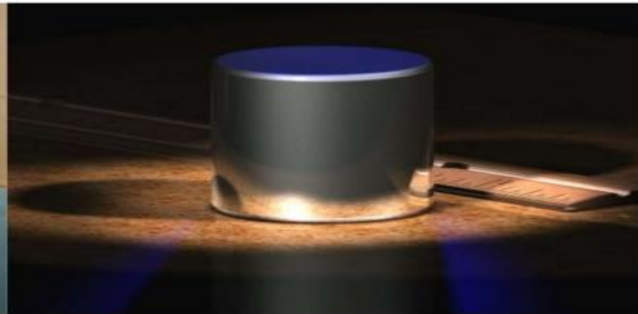
Prototype cylinder of platinum-iridium alloy
