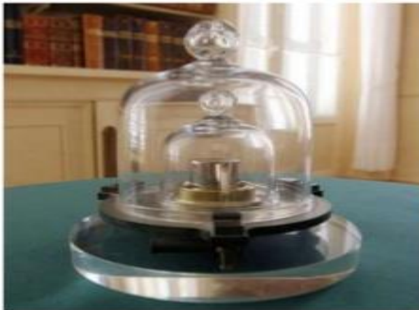
Prototype cylinder of platinum-iridium alloy
